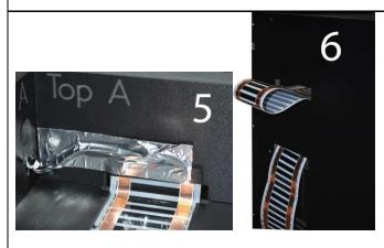
8. Probe placement: We recommend installing the thermostat probe on a center shelf as close as possible to heat tape. You may need to adjust up or down a shelf to suit your needs. Cover the probe wire (not probe tip) with 2" piece of aluminum tape. Do not cover probe tip. (Fig. 9) IMPORTANT: On back of rack use a 4" piece of aluminum tape to secure the probe cord as a strain relief.(Fig. 10)
